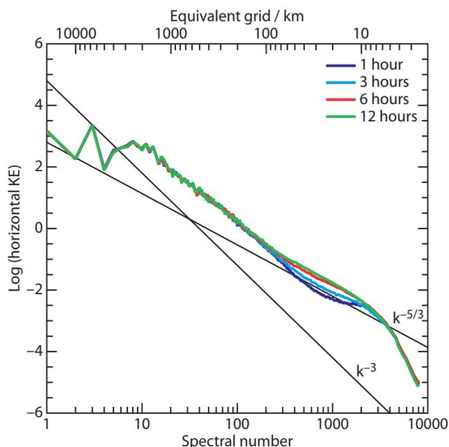
**Figure 2** Global horizontal kinetic energy spectra at 500 hPa height for the first 12 hours of the T7999 (~2.5 km grid length) simulation against the total wavenumber (with the largest number corresponding to the truncation limit of the spherical harmonics series expansion, i.e. 7999).
