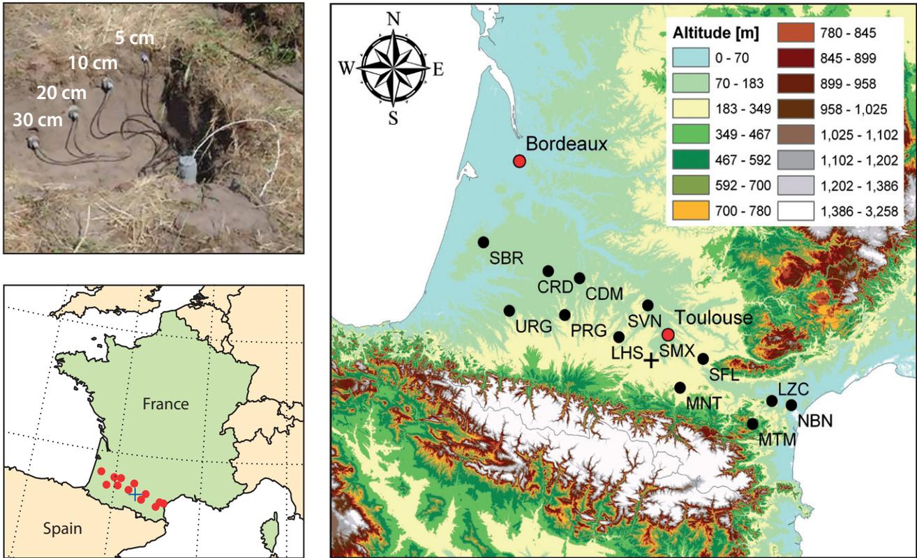
**Figure 2** Illustration of the SMOSMANIA network (from Météo-France). In-situ soil moisture measurements from this network were used to evaluate various ECMWF’s soil moisture analyses. The digital elevation model (90 m) is from the Consortium for Spatial Information (CGIAR-CSI), <http://srtm.csi.cgiar.org>. The SMOSMANIA network used ThetaProbe ML2X of Delta-T Devices.
