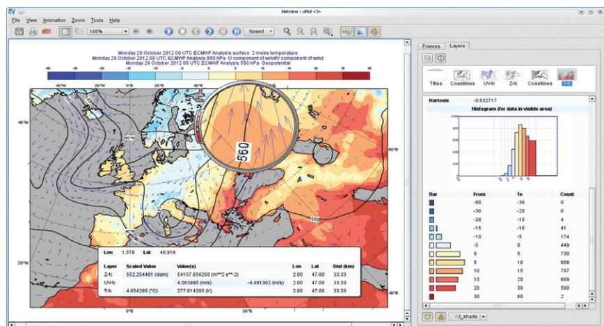
**Metview's interactive display window.** The screenshot shows plots and statistics for model fields of 2-metre temperature, 850 hPa wind and 500 hPa geopotential.
