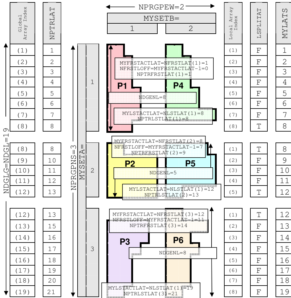
Figure 2.3 Variables describing the Grid Point Decomposition.
