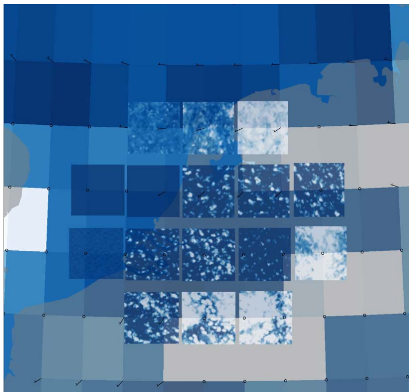
Snapshot showing liquid water path, from a preliminary test run with OpenIFS on a T255 grid, coupled to 16 DALES instances placed over the Netherlands.
